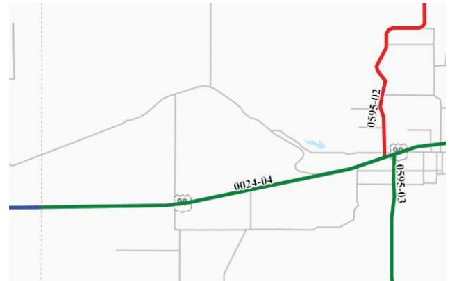
Example from Statewide Planning Map showing CS of current US 90 alignment. Use that CS (0024-04) to research as-built historic plans.
