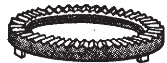
Serrated Locking Ring-Detail
