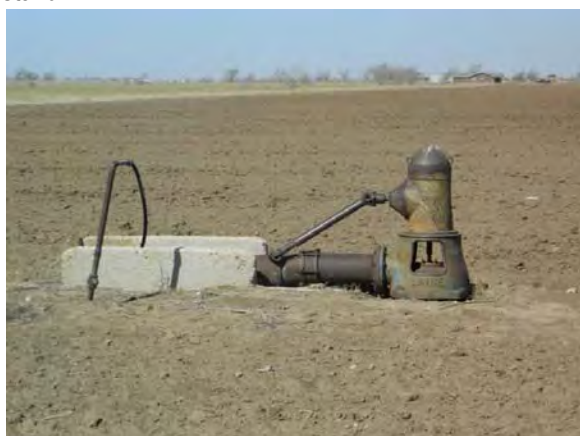
Figure F-6: Typical irrigation pump and concrete engine stand. Figure F-7: typical well house and pump.
