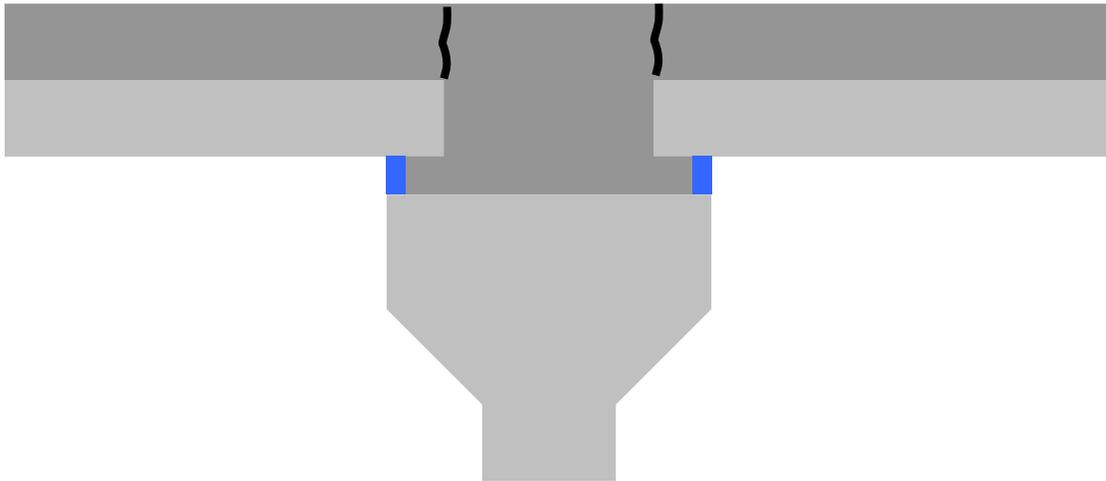
Fig. 12 Longitudinal Cracks over Girders
