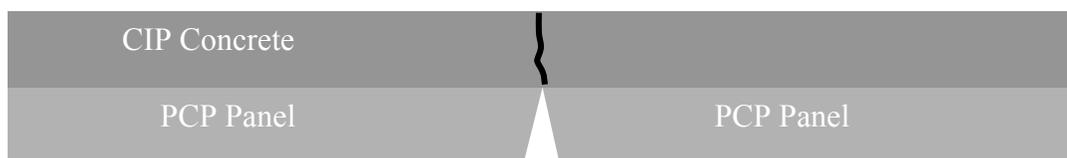
Fig. 13 Transverse Cracks between Panels
