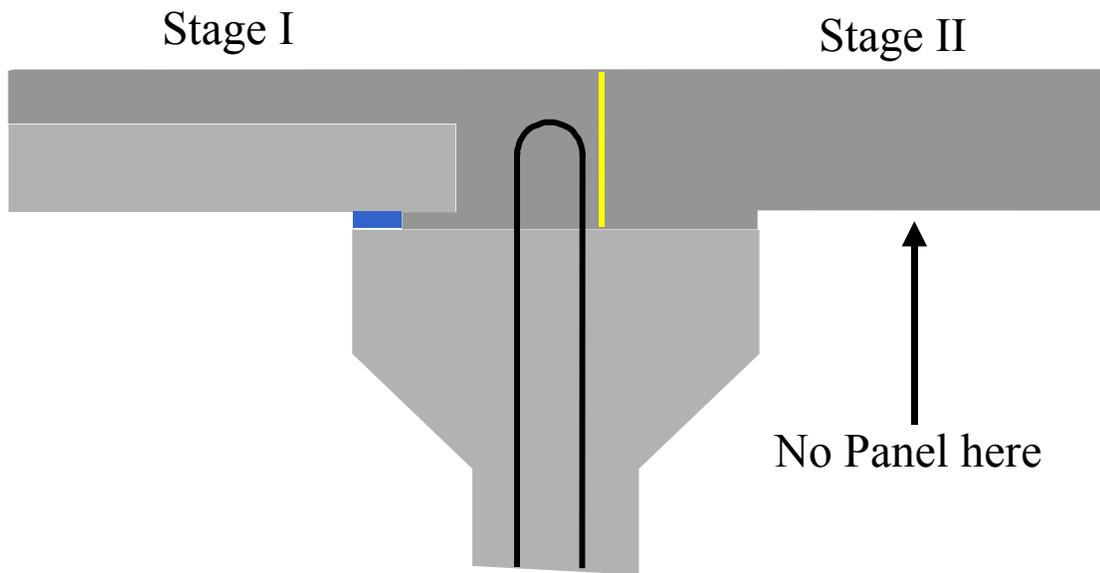
Fig. 3 Standard PCP Installation for Phased Construction
