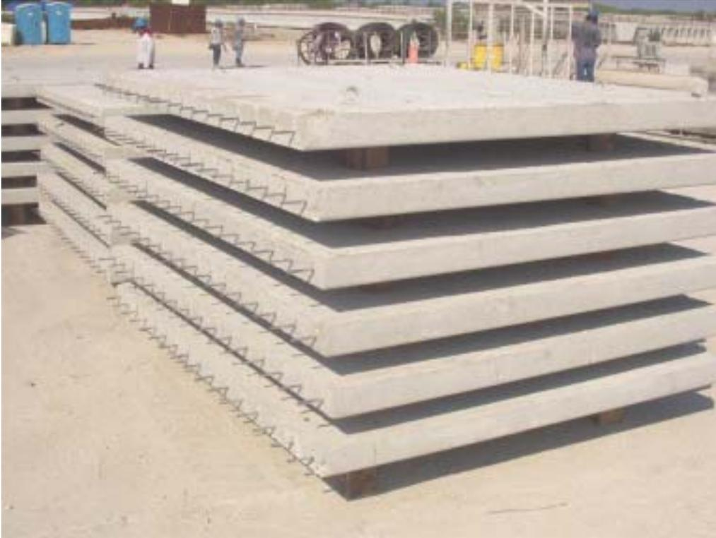
Fig. 6 Completed Panels in Storage – Note 3” Strand extension
