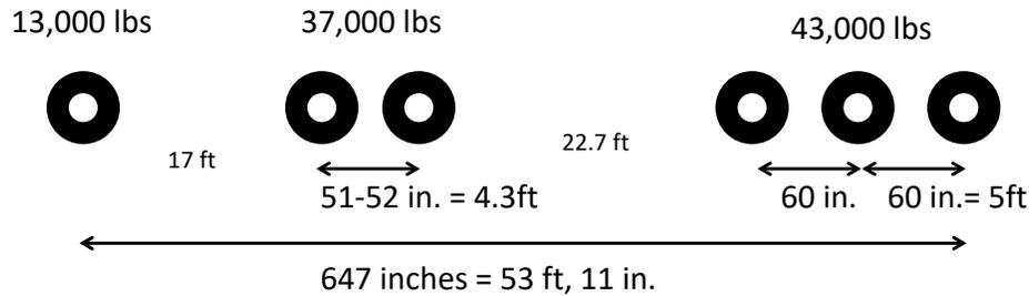
**Figure 2: HB2319 Vehicle Configurations for the Bridge Consumption Analysis**
