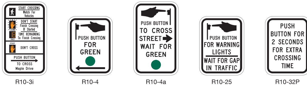
Figure 2B-27. Pedestrian Signs and Plaques (Sheet 2 of 2)
