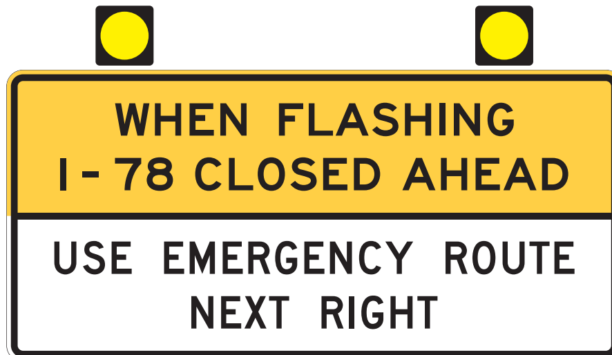
Example of advance sign for rerouting
