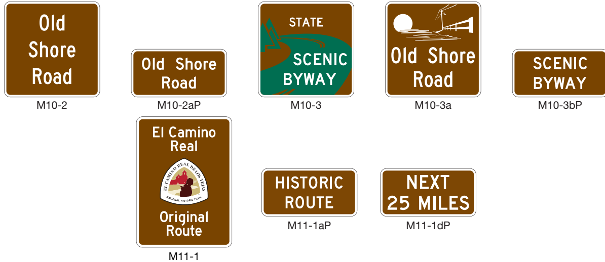
A – Byway Identification, State Scenic Byway, and National Historic Trails signs and plaques
