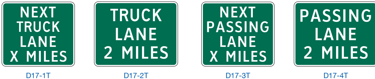
Figure 2D-25. Truck and Passing Lane Signs
