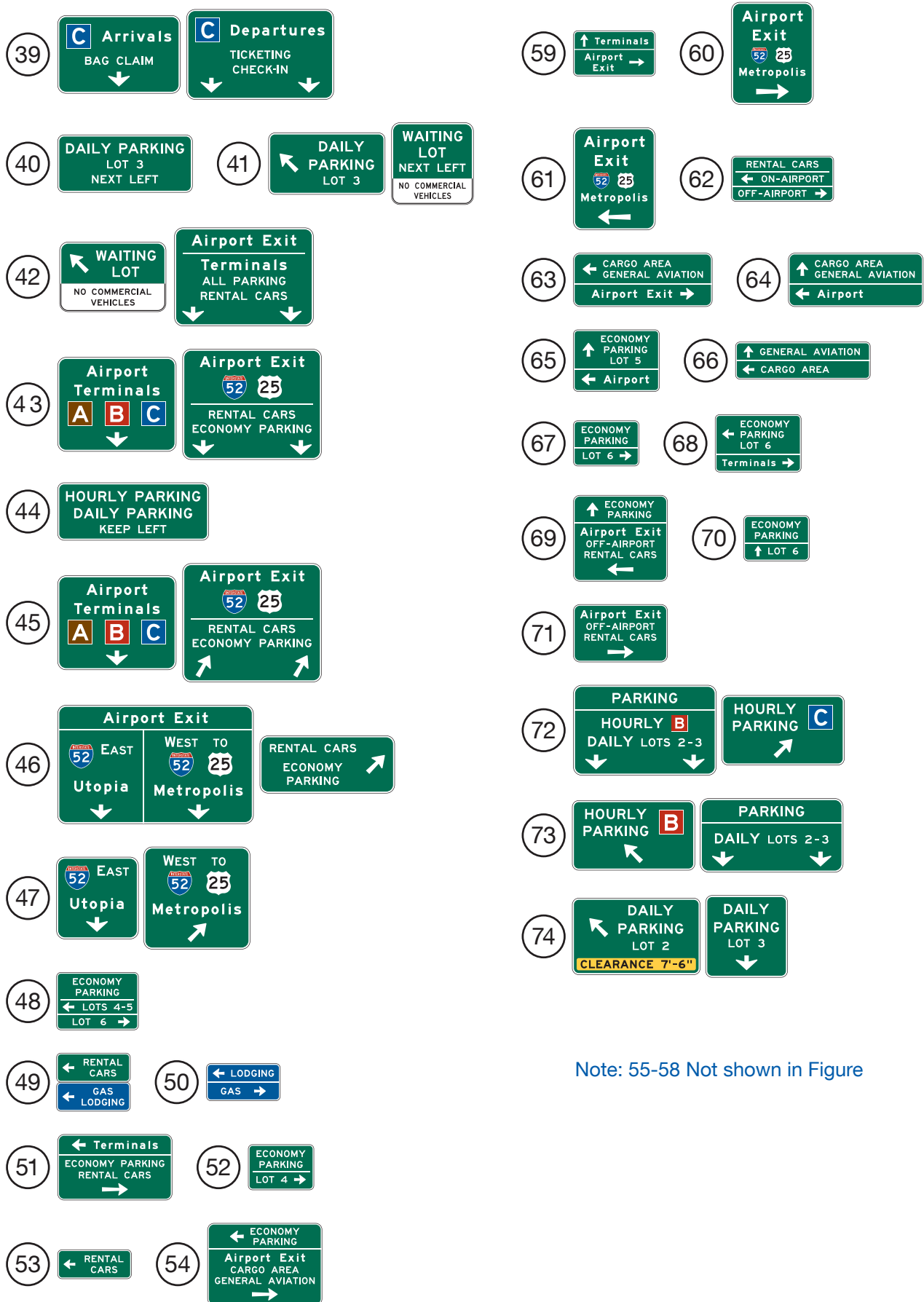
Figure 2D-39. Example of a System of Major Guide Signs for an Airport Roadway Network (Sheet 3 of 3)
