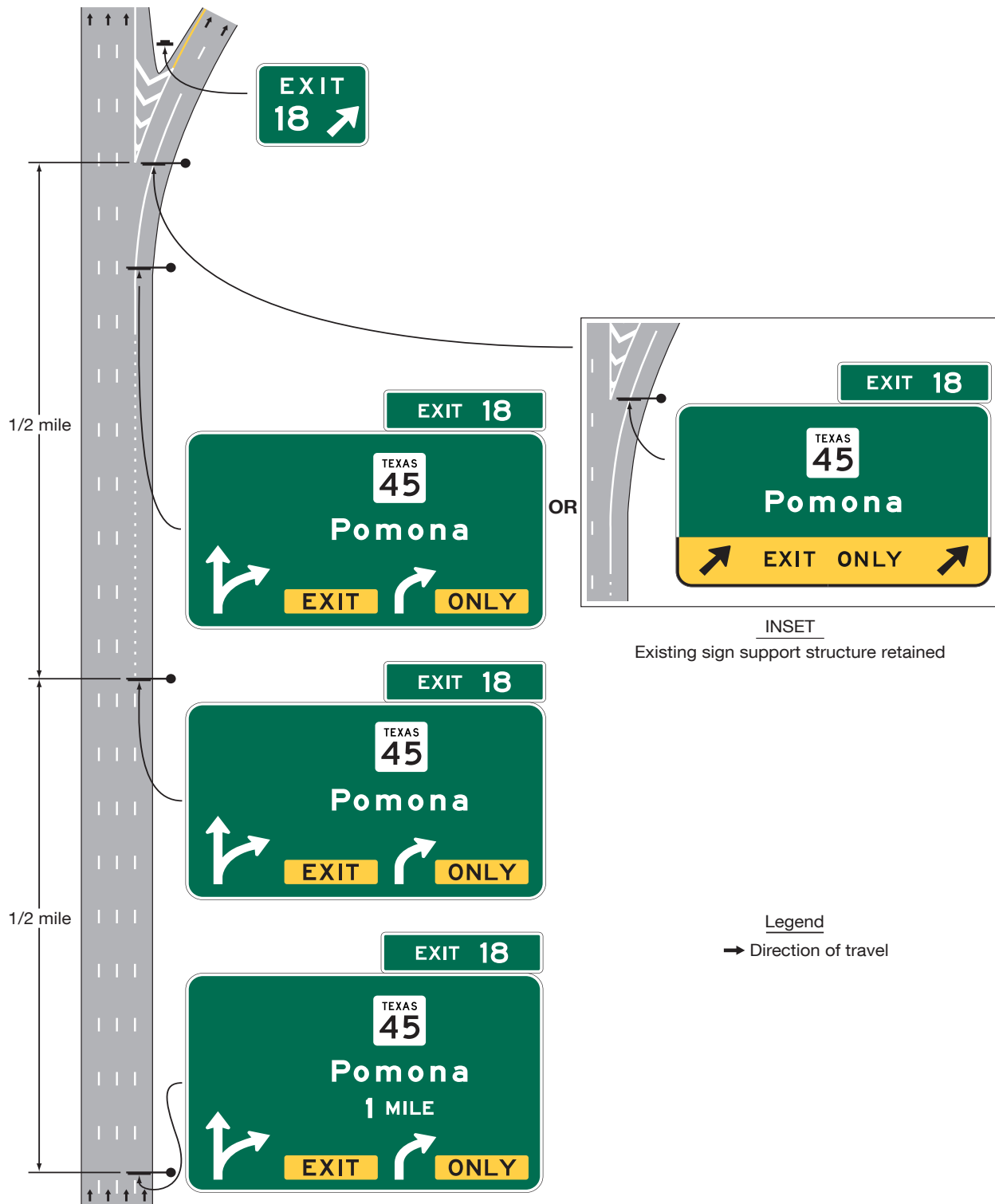
Figure 2E-44. Example of Signing for a Two-Lane Intermediate or Minor Interchange Exit with an Option Lane and a Dropped Lane using Partial-Width Overhead Arrow-per-Lane Signs
