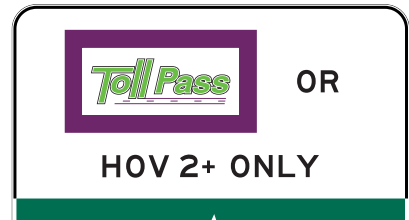
3. Pictograph with a purple underlay panel on a white or other contrasting background
