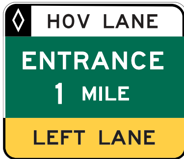
Figure 2G-5. Example of an Overhead Advance Guide Sign for a Preferential Lane Entrance
