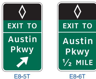
Figure 2G-12. Examples of Barrier-Mounted Guide Signs for an Intermediate Egress from Preferential Lanes
