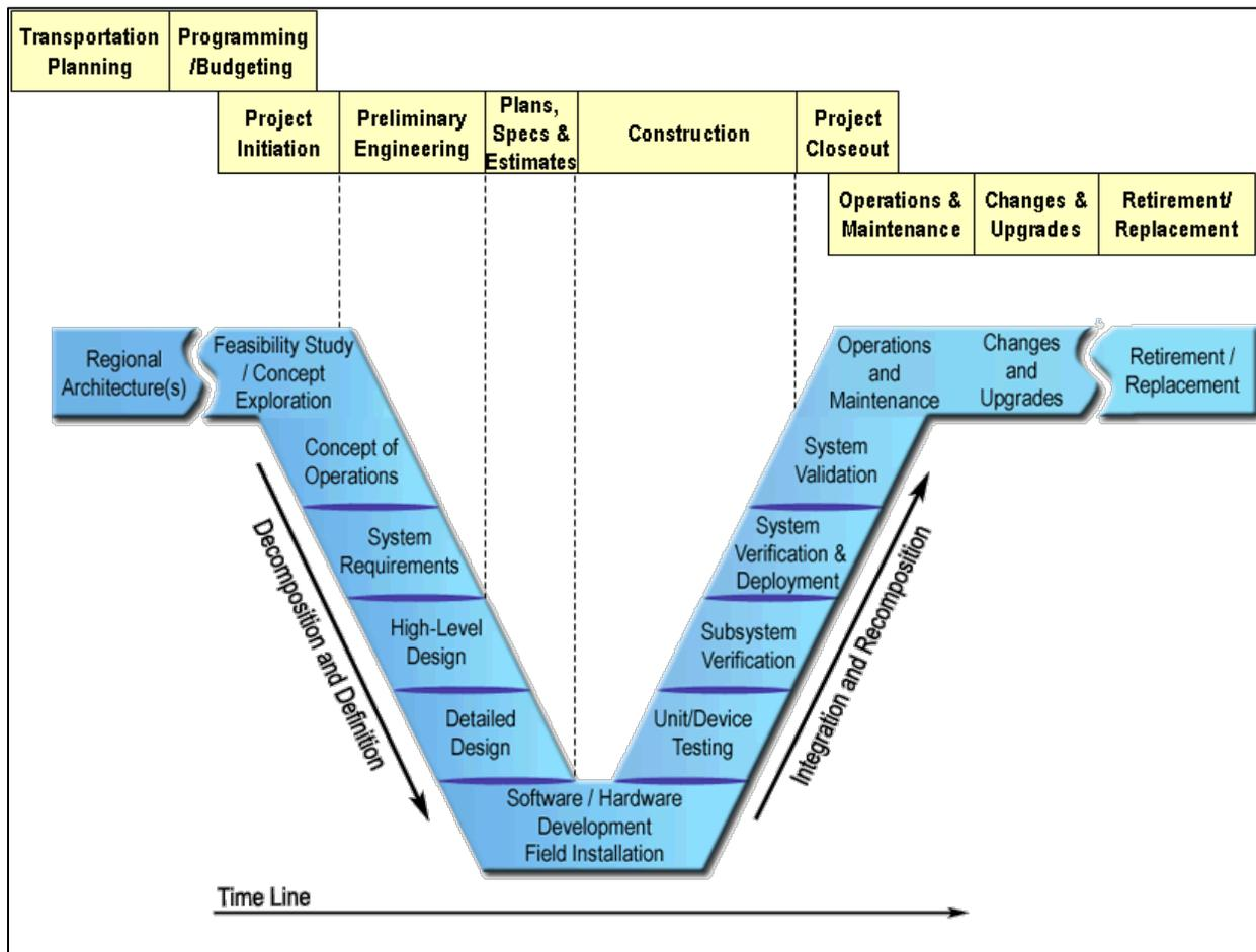
Figure 2: FHWA Systems Engineering Process “V” Diagram
