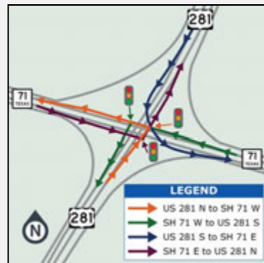
Alternative 3: 3-Level Diamond with South-to-East Flyover
