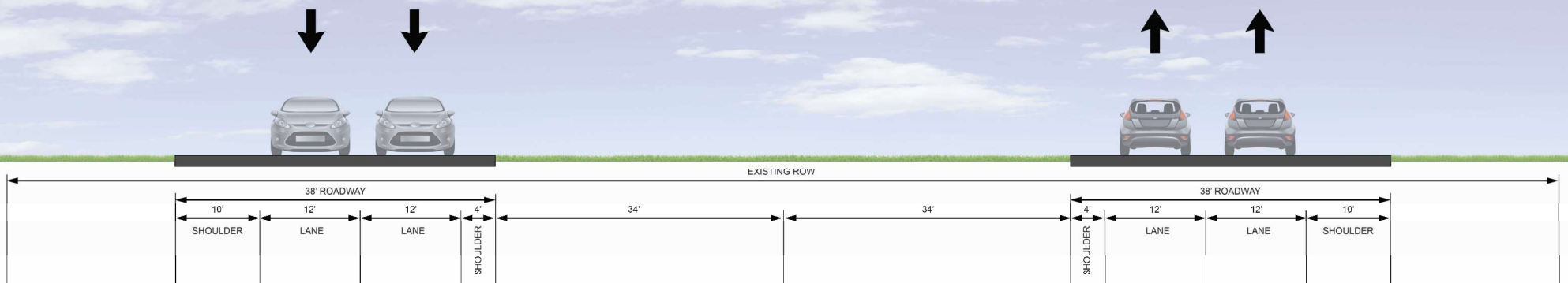
SH 47 EXISTING TYPICAL SECTION
