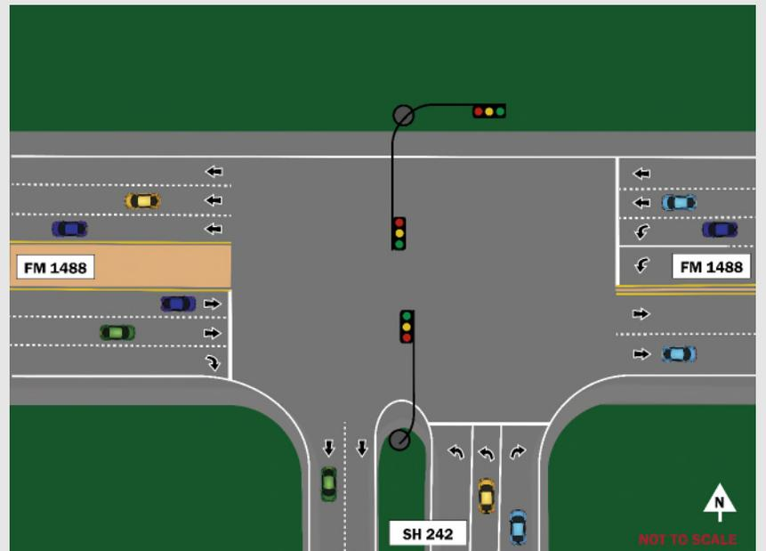
This project proposes to widen the pavement on the north side of FM 1488 between State Highway 242 and Kuykendahl. This widening would allow for the addition of a westbound auxiliary lane and an extra left turn lane at each intersection with the purpose of alleviating traffic congestion at those major intersections.
