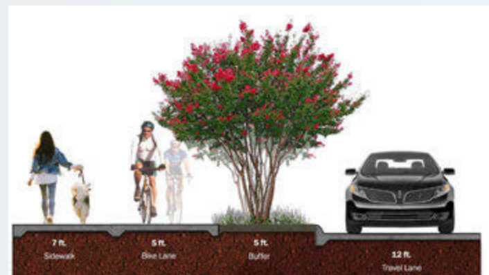
Artistic rendering depicts one-way elevated bike lane behind the curb with buffer between pedestrians and bikes, allowing for tree plantings. Illustration is not to scale and is subject to change.
