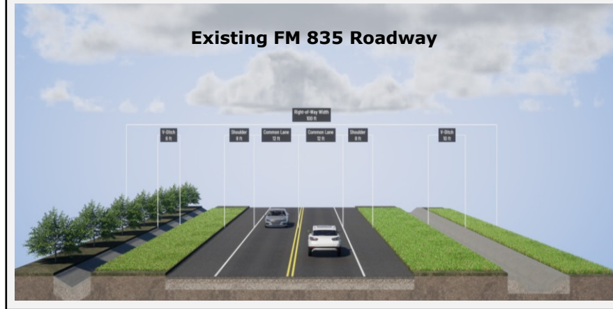
The existing FM 835 roadway approaching the bridge has 12-foot travel lanes, 8-foot shoulders and concrete riprap for drainage.
