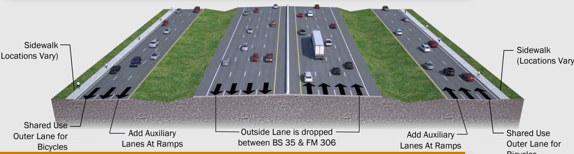
Proposed Guadalupe River to Kohlenberg Rd/Conrads Ln 6 Main Lanes and One-Way Frontage Roads
