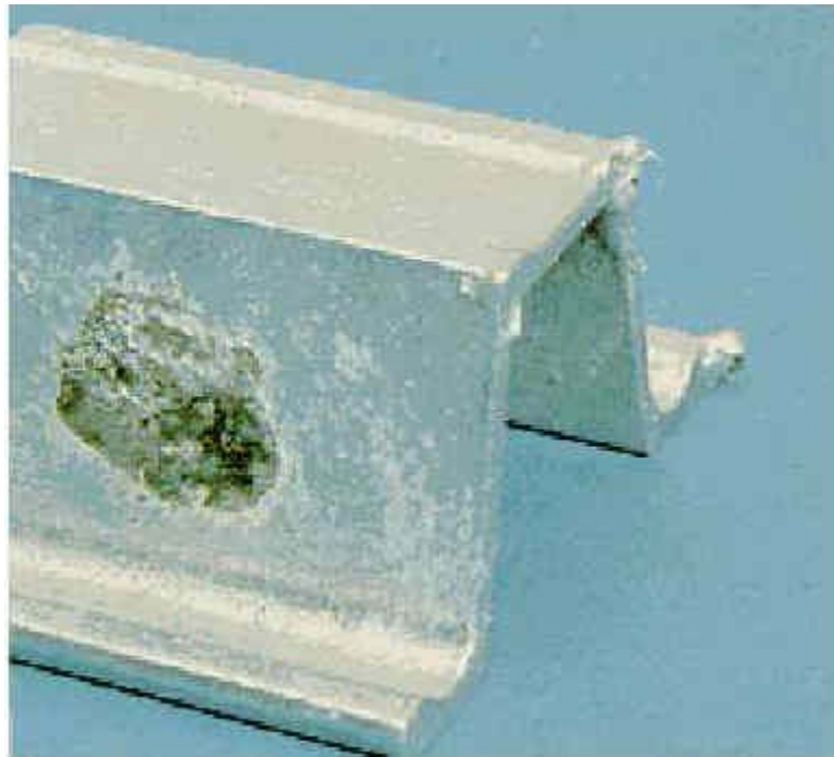
Figure 32-2—Bare (Ungalvanized) Area
