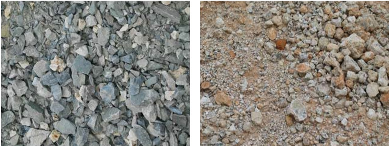
Figure A 5 - Base Material after Tested with Wet Ball Mill (Left: Granite, Right: Caliche)
