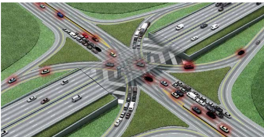
Lastly, traffic on the second set of opposing left-turn lanes travels from the cross street onto the frontage road. Through-traffic on the frontage road is handled via an intersection bypass lane, which allows vehicles to avoid the traffic signal.
