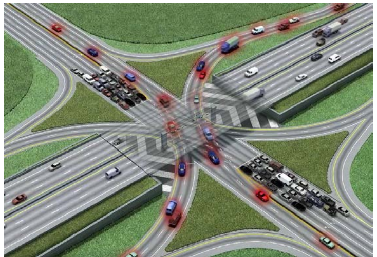
Second, traffic on the first set of opposing left-turn lanes travels through the same signal from the frontage road onto the cross street.
